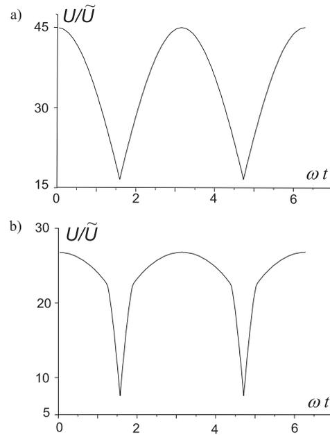
**Figure 3.** The time dependence of the voltage  $U$  at relatively small ((a)  $h_m < H$ ) and large ((b)  $h_m > H$ ) AC amplitudes.
