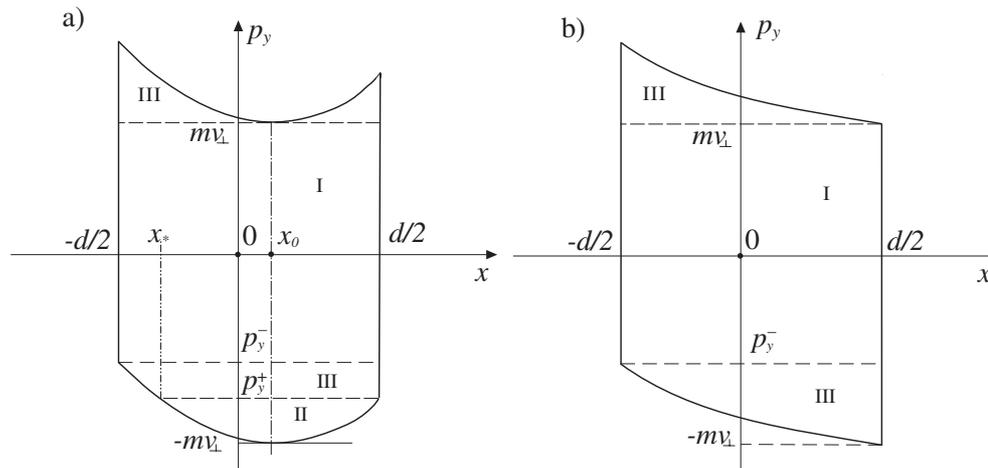
**Figure 2.** The phase space  $(p_y, x)$ . Regions of existence of flying (I), trapped (II), and surface (III) particles in a spatially sign-alternating (a) and a constant-sign (b) total magnetic field.
