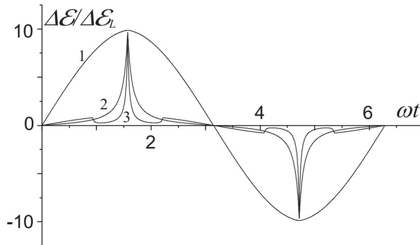
**Figure 4.** The dependence  $\Delta\mathcal{E}(t)$  for  $H = 300\tilde{H}$  and various amplitudes of the AC signal:  $h_m = 1\tilde{H}$  (1),  $h_m = 200\tilde{H}$  (2),  $h_m = 500\tilde{H}$  (3). The ratio of the mean free path  $l$  to the film thickness  $d$  equals 30.
