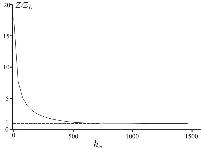
**Figure 5.** The surface impedance  $Z$  (in units of the impedance  $Z_L$  in the absence of the direct current) versus the dimensionless amplitude  $h_m/\tilde{H}$  of the AC signal at  $H = 500\tilde{H}$ .
