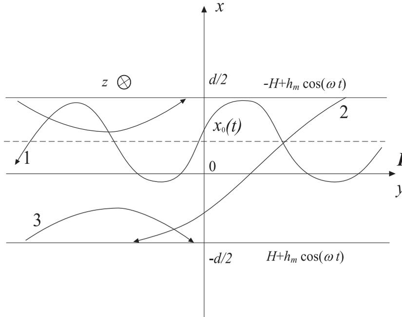
**Figure 1.** The geometry of the problem. A schematic representation of the trajectories of trapped (1), flying (2), and surface (3) electrons.
